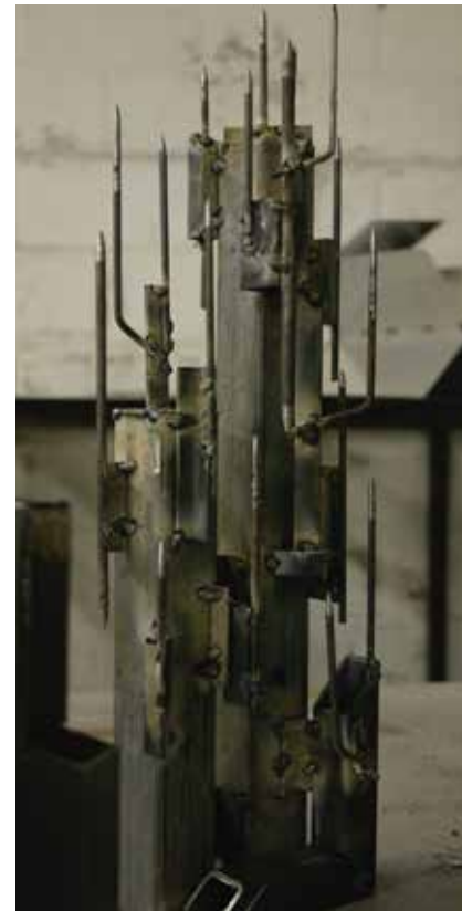
The buildings were first roughed out in welded steel. This allowed for oven-bake sculpy to be spread over the entire surface for sculpting.
